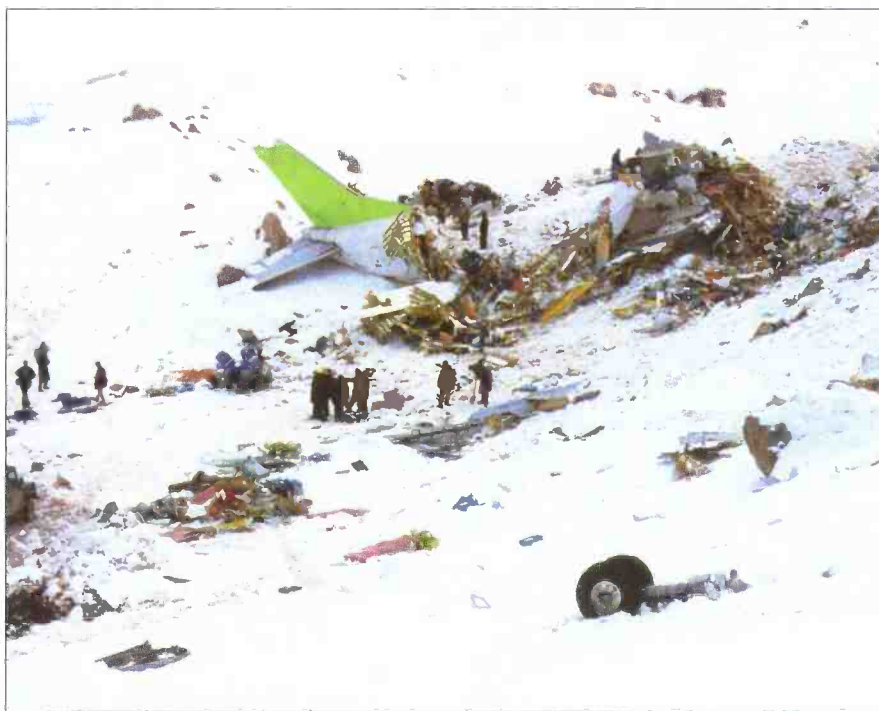
Figure 12. This accident site, the same as shown on page 1, is on a downslope just four miles from the intended landing runway. The airplane was experiencing gusty winds and heavy snow, and was at an altitude well below approach minimums when it hit the mountain.
