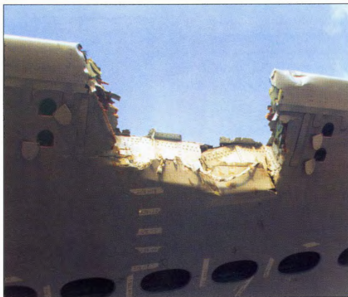
Figure 7. While most CFIT incidents and accidents occur during approach and landing, this shows what can happen during departure. In this incident, a 767 struck the very top of the communication tower shown on the left. The damage to the wing, shown in the photo above, is what resulted. The crew was able to safely return to the departure airport.
